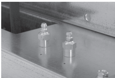
External Grease Fittings
