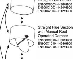
Straight Flue Section with Manual Roof **Operated Damper**
